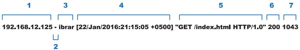
Fig. 1. Format of an access log file.
