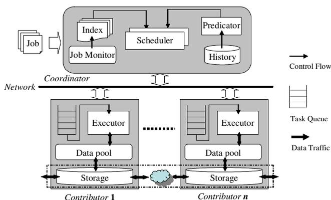
Figure 1 Architecture of Dataflow System
