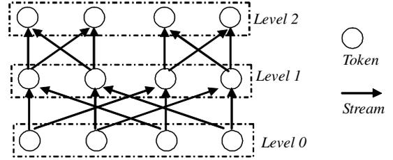
Figure 2 Dataflow graph of FFT with 4 points
