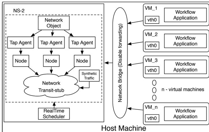
Figure 7: Experiment design using NS-2 based emulation
