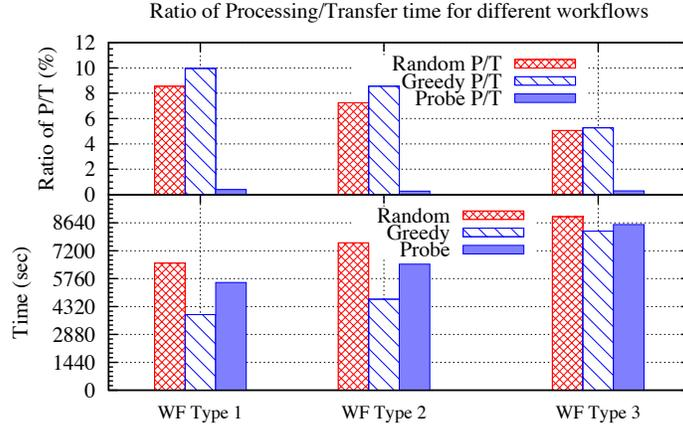
Figure 10: Average data transfer and segment-processing times of all files using random, greedy and probe-based retrieval techniques for three workflow (WF 1, WF 2 and WF 3 corresponding to Montage, LIGO and IR workflows in Figure 6)
