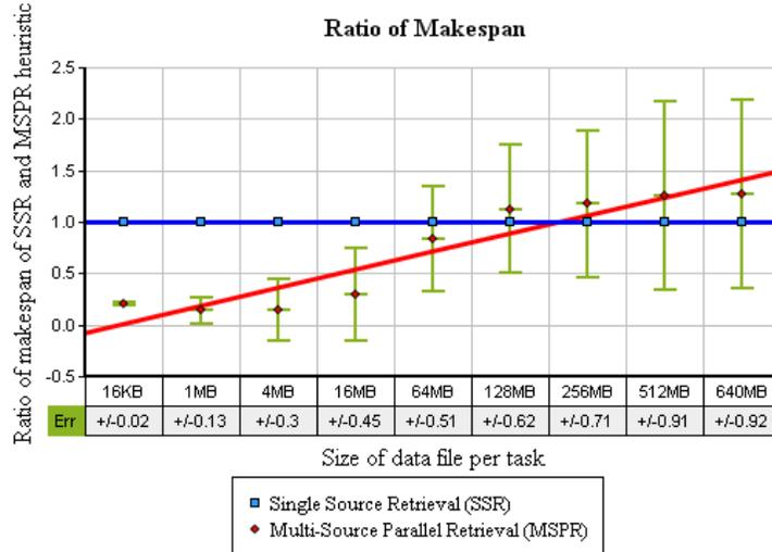
Figure 13: Determining the benefit of using multi-source parallel data retrieval by comparing the ratio of makespan for IR workflow (WF type three) in real environment
