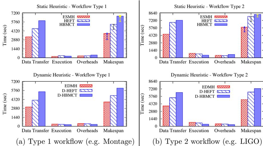
Figure 11: Makespan of Montage and LIGO (Type 1 and 2) workflows when using static and dynamic heuristic.
